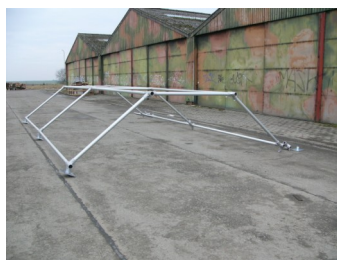
Frame made with aluminium tubes
