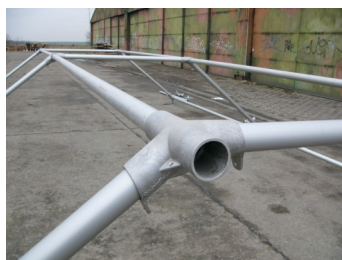
Cast aluminium corners
